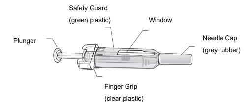
Activate the green safety guard manually (slide over the needle) after the injection.
